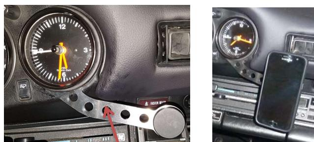
Adjust the position of the holder before pressing in the clock.
