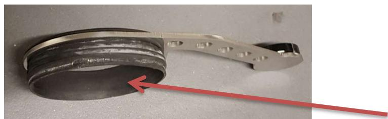
Fit the rubber clamping ring into the holder, smearing a little cream on the inside if necessary, so that it slides better over the watch case.
